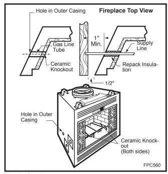
Fig. 27 Gas line access.
